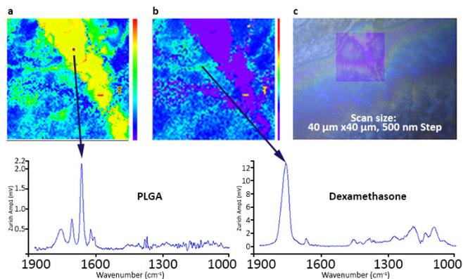
Figure 5: HYPERSpectral images and corresponding spectra taken at (a)  $1760\text{ cm}^{-1}$  showing PLGA distribution, and (b) at  $1666\text{ cm}^{-1}$  showing dexamethasone. (c) Optical view of PLGA/dexamethasone blend, with a  $40 \times 40\text{ }\mu\text{m}$  image selected for simultaneous HYPERSpectral measurements. Data courtesy of [??]
