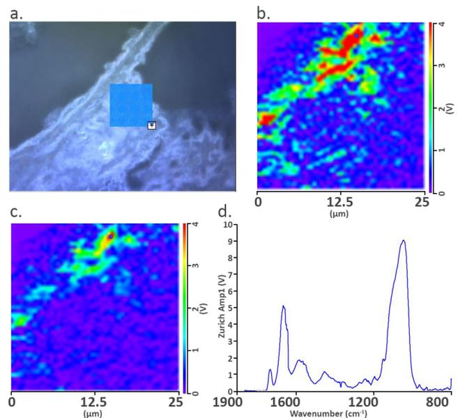
Figure 4: A. Hyperspectral array location of mouse bone. HYPERspectral images and taken at B. 1047  $\text{cm}^{-1}$  and C. 1660  $\text{cm}^{-1}$  showing mineral and protein distribution, respectively. D. Corresponding spectra taken from the inner bone, showing a higher absorption for phosphate. Data courtesy of Prof. Nancy Pleshko, Dr. Mugdha Padalkar, and Jessica M. Falcon, Temple University
