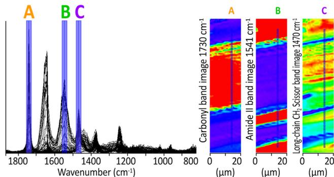
Figure 6: A block face of a multilayer polymer film sample with seven layers. HYPERSpectral images of  $20 \times 85\text{ }\mu\text{m}$  size were taken at a rate of 1 sec/spectrasize, with  $1\text{ }\mu\text{m}$  spacing. The spectra shows the corresponding spectra and images of absorption of carbonyl, amide II, and CH stretching bands of the film components, respectively. Data courtesy of G. Meyers, M. Rickard Dow Chemical Company
