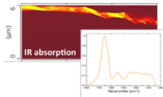
Figure 2. AFM-IR image and spectrum of individual, twisted collagen fibril. Unwound fibril thickness  $\sim 100$  nm.<sup>2</sup>
